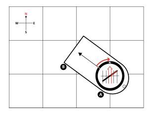
3. Hold compass level at waist height and turn yourself until the needle and orienting arrow are aligned. NOTE: Compensate for declination. See section 5.
