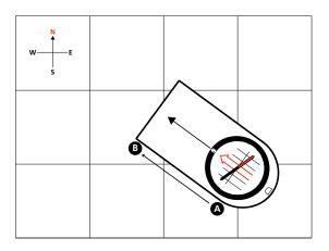
2. Turn the capsule until the orienting lines are parallel to the meridian lines on the map with N pointing north.
